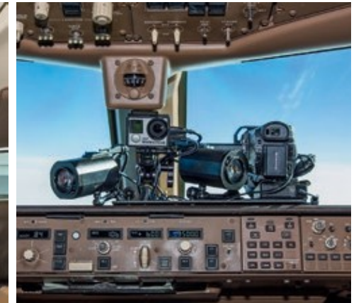
Four cameras are installed close together in front of the pilots
